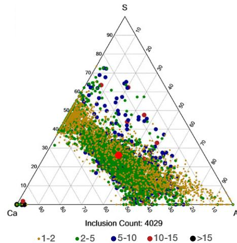
Figure 1. An inclusion population for an Al-killed, Ca-treated steel contains many calcium sulfides (left axis), calcium aluminates (center), and spinel inclusions in this 50 mm<sup>2</sup> scan.
