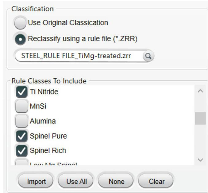
Figure 6. Snapshot of Perception Reporter Software shows that inclusion types may be incorporated in a table, chart, or ternary diagram by selecting the desired classes.
