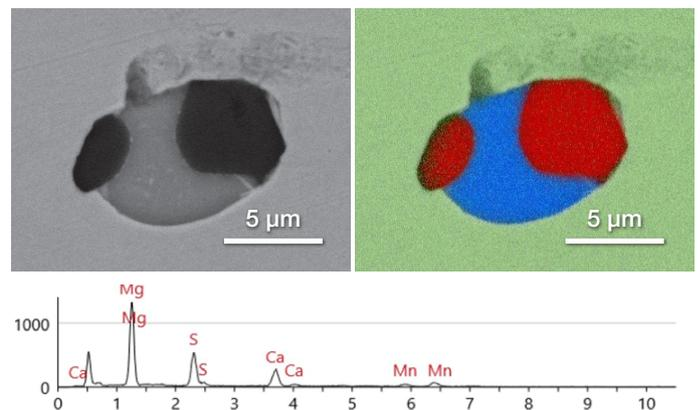
Figure 5. Manual analysis of a compound MgO-CaS inclusion showing the BSE image (left), EDS map (right), and inclusion spectrum (bottom). The map shows Mg in red and Ca in blue with a background of Fe in green.
