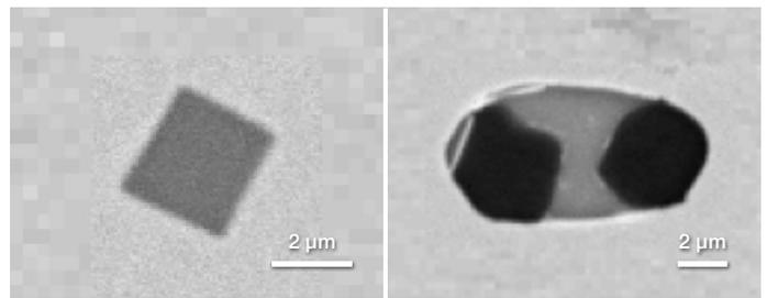
Figure 4. Backscattered electron images can be saved for every inclusion. Here, we show images of a TiN cube (left) and compound MgO-CaS (right), with MgO having a much darker backscattered electron video level. The scale bars are both 2 μm long.
