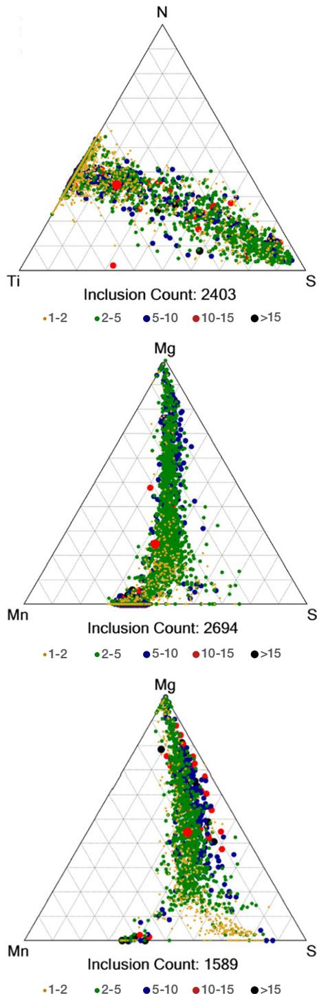
Figure 3. Ternary diagrams of Ti-S-N (top) and Mn-S-Mg (middle) after alloy additions of titanium and magnesium, and Mn-S-Mg (bottom) after calcium addition in the RH degasser.
