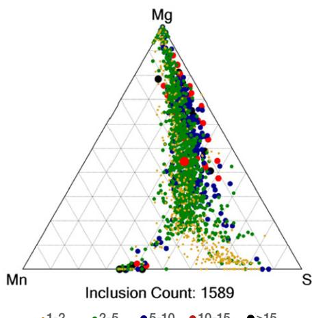
Figure 3. Ternary diagrams of Ti-S-N (top) and Mn-S-Mg (middle) after alloy additions of titanium and magnesium, and Mn-S-Mg (bottom) after calcium addition in the RH degasser.
