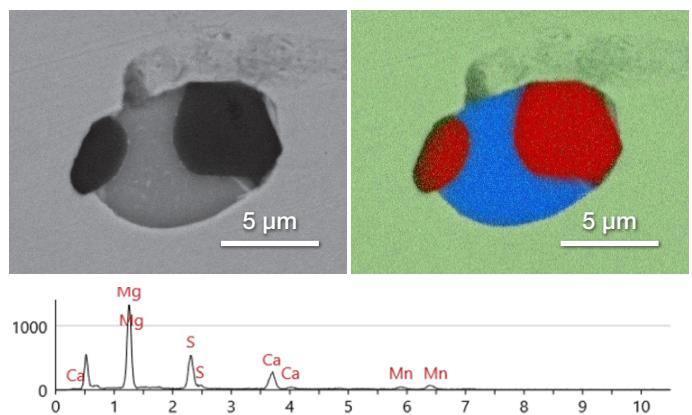
Figure 5. Manual analysis of a compound MgO-CaS inclusion showing the BSE image (left), EDS map (right), and inclusion spectrum (bottom). The map shows Mg in red and Ca in blue with a background of Fe in green.
