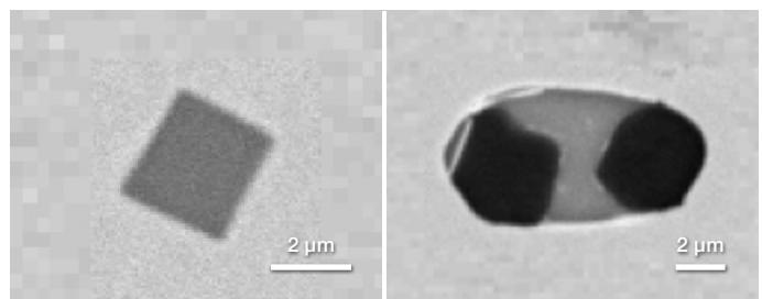
Figure 4. Backscattered electron images can be saved for every inclusion. Here, we show images of a TiN cube (left) and compound MgO-CaS (right), with MgO having a much darker backscattered electron video level. The scale bars are both 2  $\mu\text{m}$  long.
