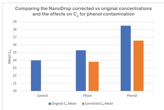
**Figure 4: The effect on C<sub>q</sub> mean results for phenol-spiked RNA samples using the corrected and original, uncorrected RNA concentration provided by the Acclaro Software. The blue bar represents the C<sub>q</sub> mean results using the original concentration. The orange bar represents the C<sub>q</sub> mean results using the corrected concentration provided by Acclaro analysis.**
