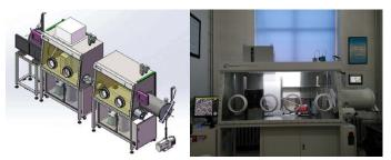
Figure 1. Left: schematic of workflow incorporating a Phenom XL G2 Desktop SEM inside a glove box. Right: actual setup of Phenom Desktop SEM inside argon filled glove box.
