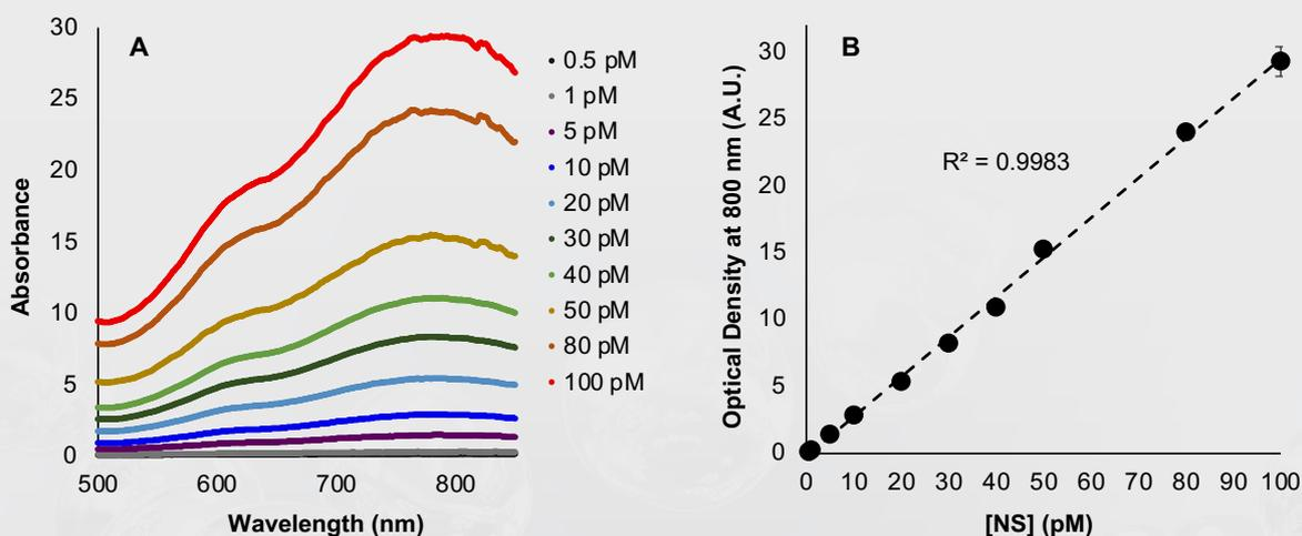
Figure 1: (A) UV-Vis spectra for 150 nm NS at concentrations ranging from 0.5 pM to 100 pM, as measured on the NanoDrop One Spectrophotometer. (B) The OD of NS at 800 nm as measured by the NanoDrop One Spectrophotometer plotted versus known concentration, showing a linear relationship over a large range of 0.5 pM to 100 pM with an  $R^2$  value of 0.9983.  $n=3$ .
