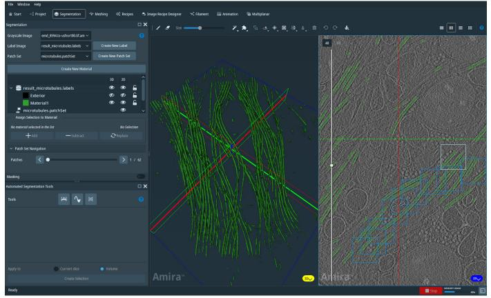
Figure 4. AI-assisted segmentation in the Segmentation+ workroom.
