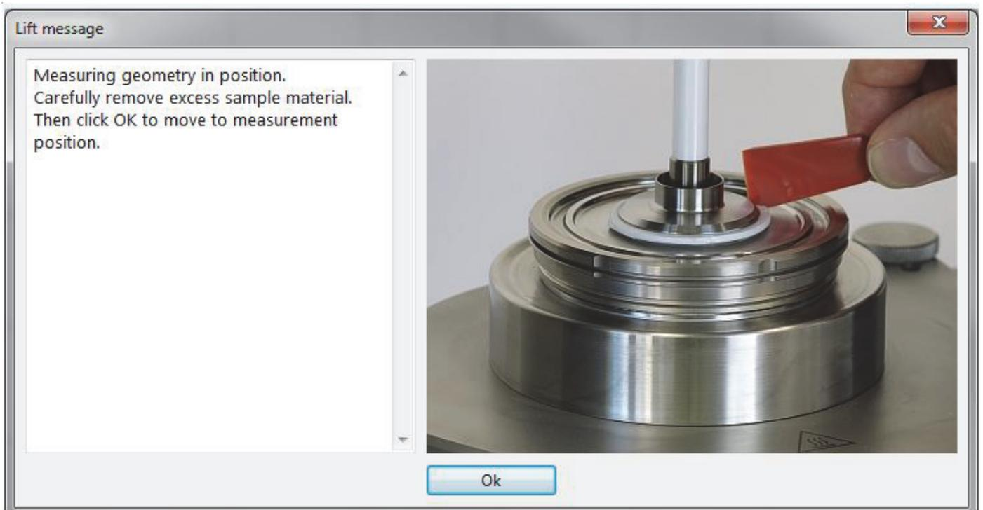
Fig. 6: HAAKE Rheowin software sample trimming message.
