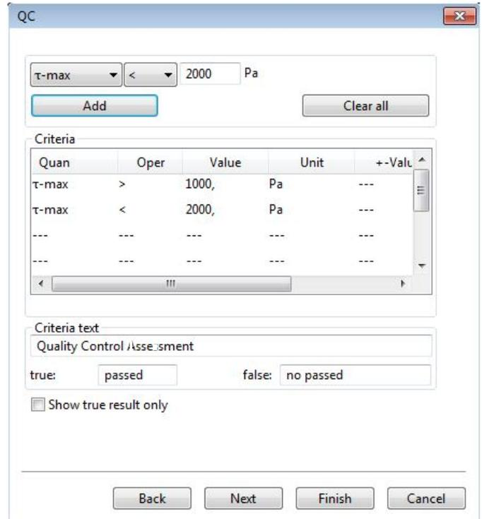
Fig. 7: Definition of QC criteria in HAAKE RheoWin software.
