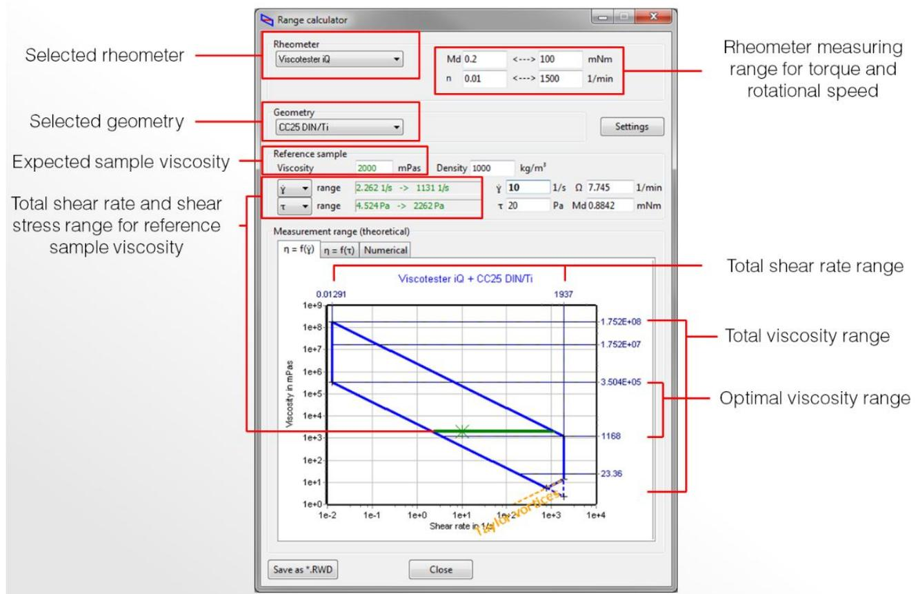
**Fig. 2:** HAAKE RheoWin software range calculator tool.
