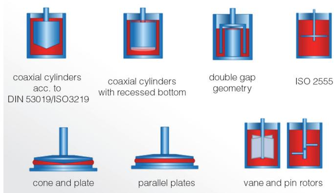
Fig. 1: Overview of standard measuring geometries.
