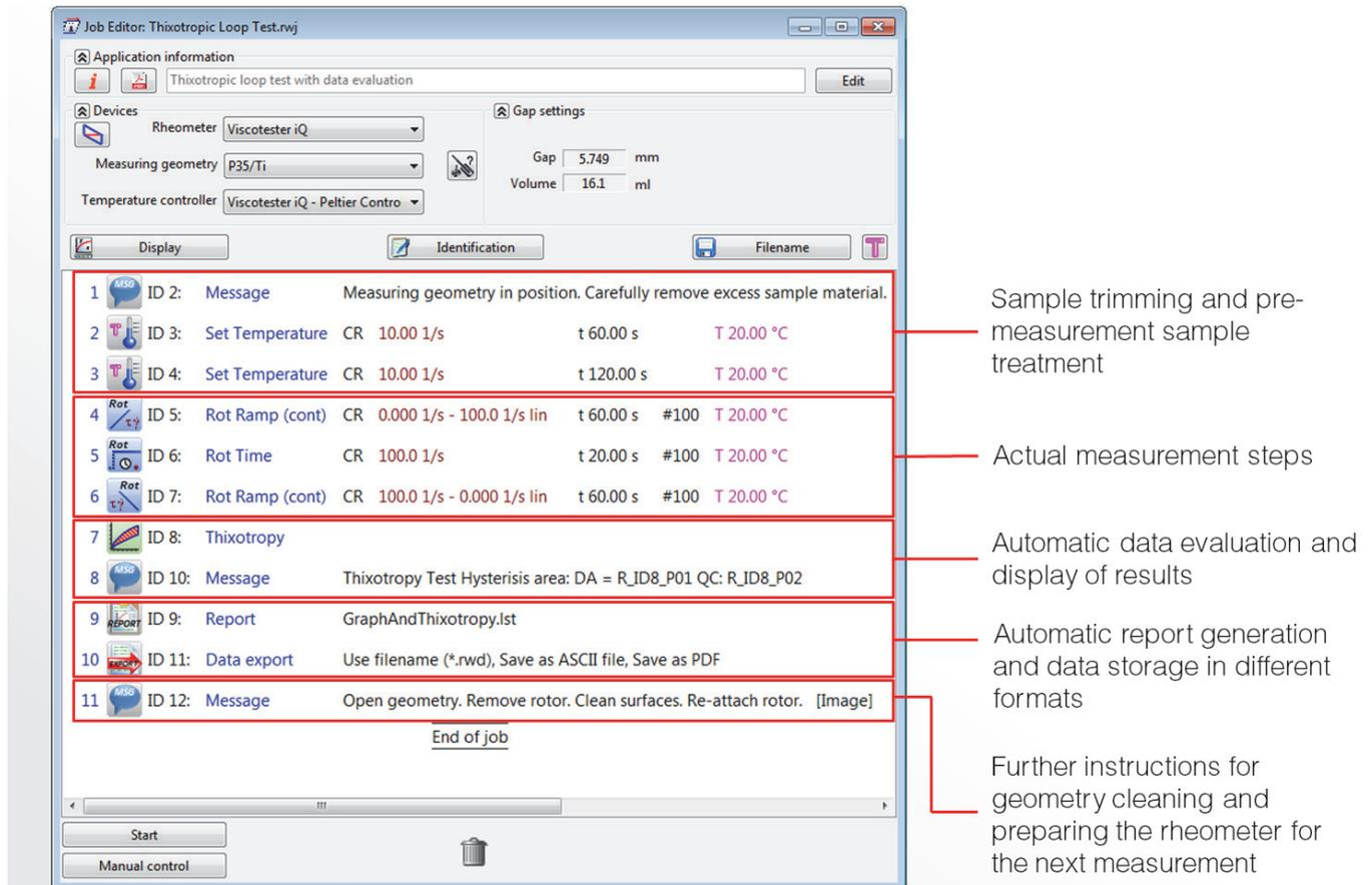
Fig. 8: Complete HAAKE RheoWin software test procedure.
