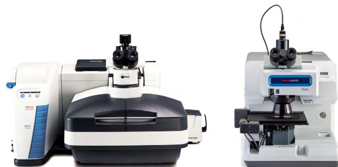
DXR3xi Raman Imaging Microscope and Nicolet RaptIR FTIR Microscope.
