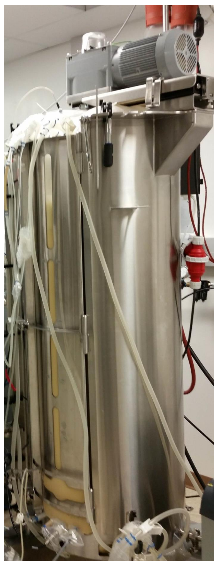
Figure 2. 300 L culture at 600 slpm gas flow and 375 rpm.
