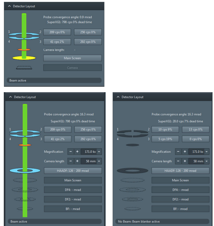
Figure 4: Example of interactive detector layout. The active detectors are indicated (light blue). The examples show SmartCam imaging (top), STEM HAADF imaging (bottom left), and a blanked beam condition (bottom right).
