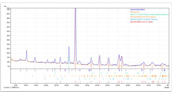
N.R.: The largest peaks with red vertical sticks are all Calcite = Limestone. Quartz peak is identified (blue vertical stick)
