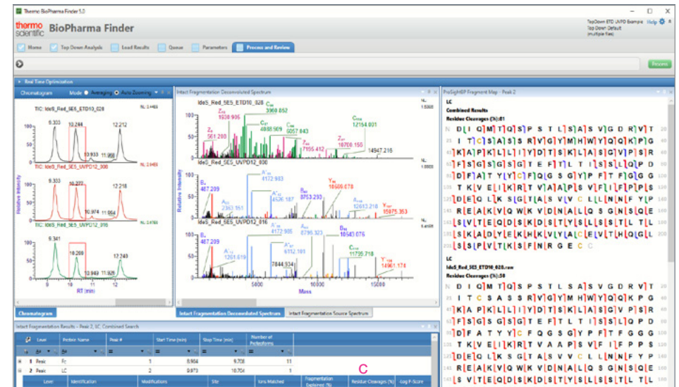
The combined search of ETD and UVPD data can be used to produce a combined coverage map displaying the dissociation type for each of the generated fragments identified.
