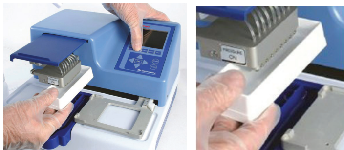
Figure 3. Cleaning dispensing valves with solution in reservoir.
