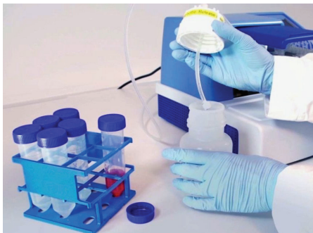
Figure 2. Inserting tubing into 50 mL conical tube.
