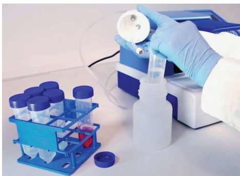
Figure 1. Inserting 50 mL conical tube into reagent vessel.
