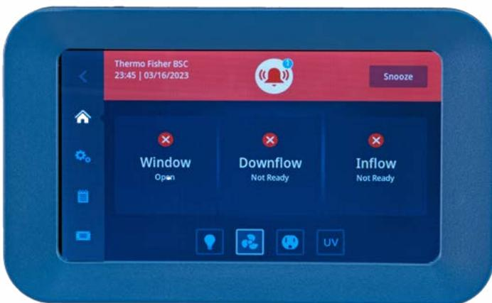
Clear visual and audible alarm are emitted from the device if the downflow, inflow, or other parameters are not at operational settings and operator is at risk of exposure to biohazardous materials.
