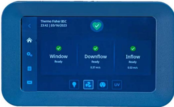
The unit is in working mode, with glass sash in its working position, and both the downflow and inflow air speeds at operational speeds. The white outline around the fan logo at the bottom means the blowers are all on.
