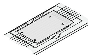
3. Slowly and steadily push the carriage across the sealer in the direction of the engraved arrows. Push the carriage across the entire length of the card until the carriage meets the mechanical stops at the ending position.
