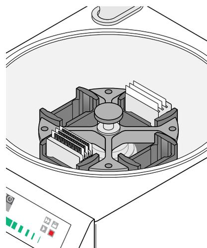
Centrifuge is properly loaded and balanced.
