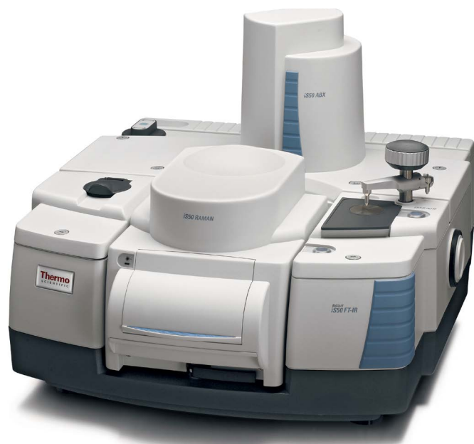
Figure 1: The Nicolet iS50 FTIR Spectrometer configured with the iS50 ABX Automated Beamsplitter exchanger, the built-in iS50 ATR module, and the iS50 Raman module
