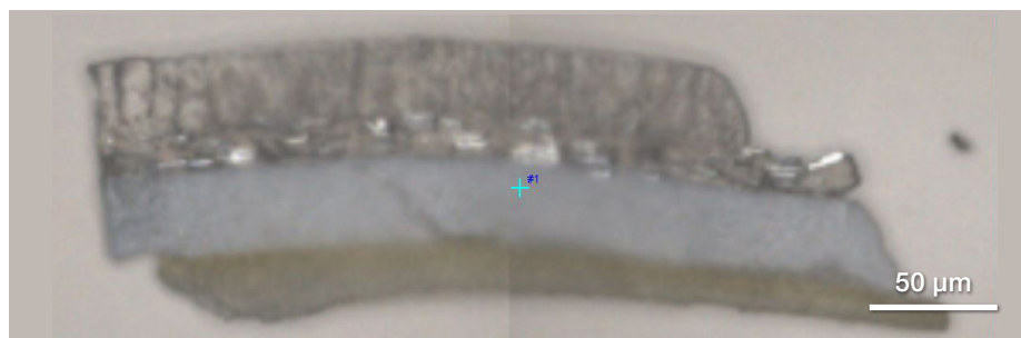
Figure 1. Schematic of a typical four-layer automobile paint sample (left). Video mosaic image of a paint-chip cross-section taken from the door of an automobile (right).
