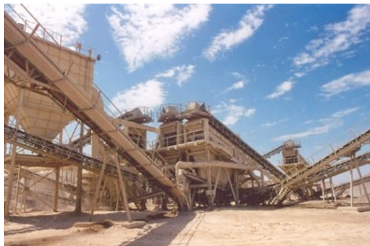
Mining Quarry: Raw materials are moved around the facility using conveyor belts
