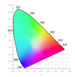
CIE Chromaticity Diagram describes colour as seen by the human eye in full daylight. Two-dimensional diagram of colours with same brightness (intensity). All colours of visible spectrum are represented.
