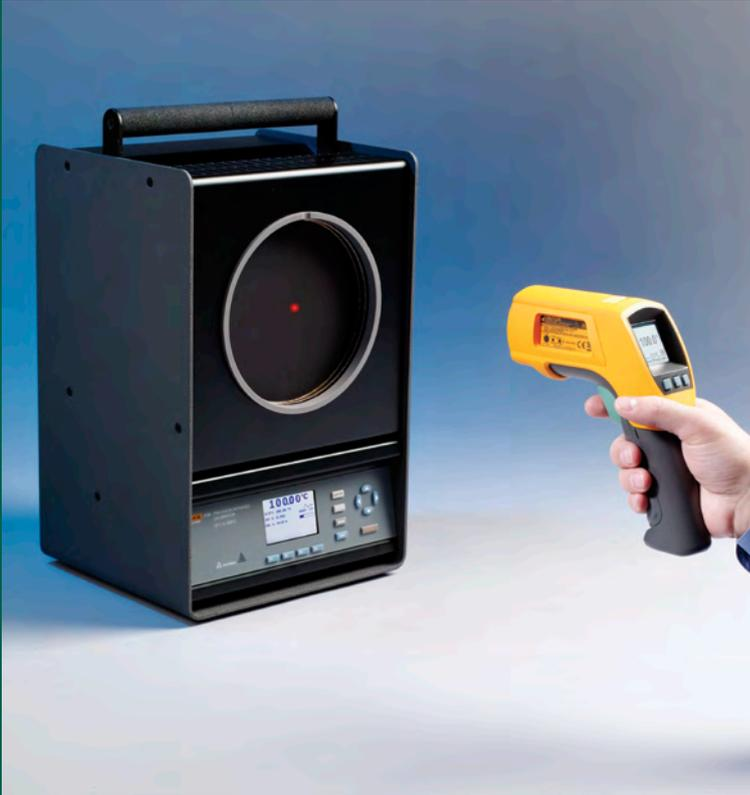
Infrared thermometer calibrations can be accurate with the proper setup and planning. It's important to choose a calibrator with a radiometrically calibrated target that is large enough to accommodate the recommended calibration distance of common infrared thermometers, along with their various fields of view.
