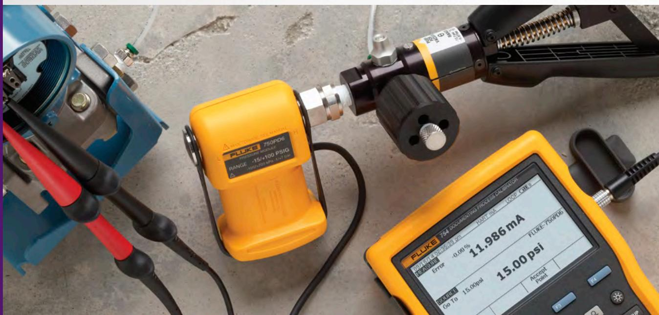
Classic methods for pressure switch testing have been superseded with the introduction of new pressure test tools. Today most pressure switches are tested with a pressure gauge mounted to a pump to supply and measure pressure, and a DMM set to continuity to verify the opening and closing of the switch. The technician or electrician making the test is required to interpret the pressure applied to the switch
