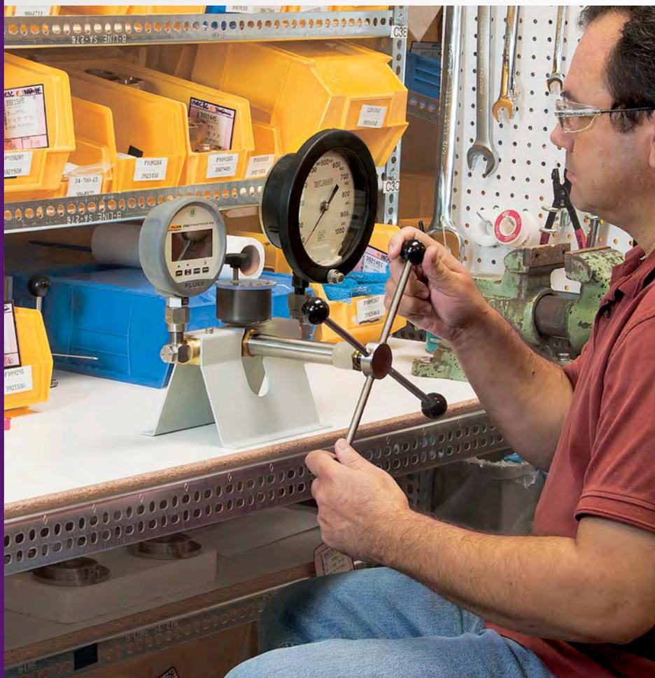
A pressure comparator is a convenient instrument for bench pressure calibration. Bench calibrations are performed to maintain reference conditions and to obtain the lowest possible uncertainties. The bench is also a convenient place to inspect, adjust, and repair the devices under test.
