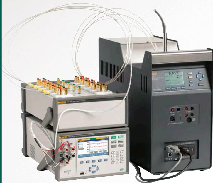
Thermocouples are common in industry because they are inexpensive and cover a wide temperature range.
