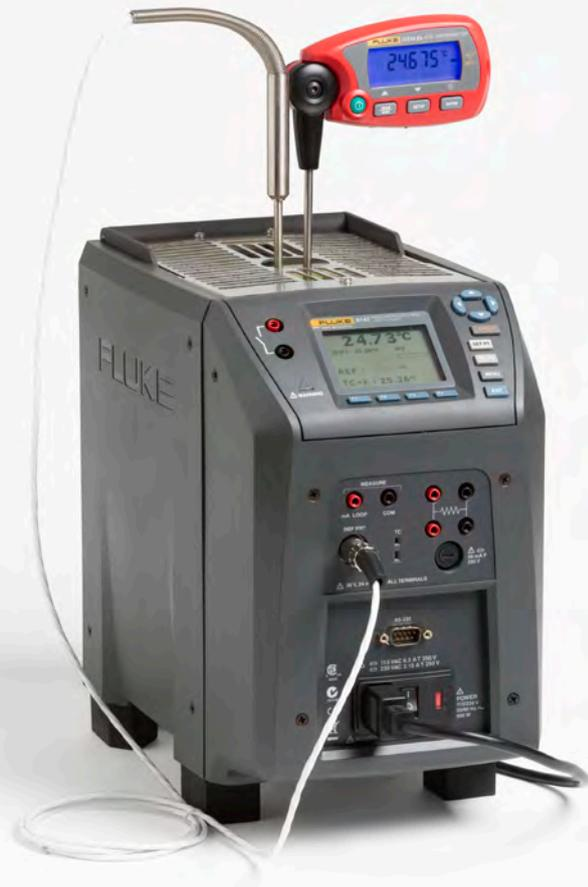
Typically RTDs are checked while calibrating the connected device, such as a panel meter or temperature transmitter. However, if a problem is suspected with a temperature sensor, sensor calibrations can be performed separately from the calibration of process electronics.
