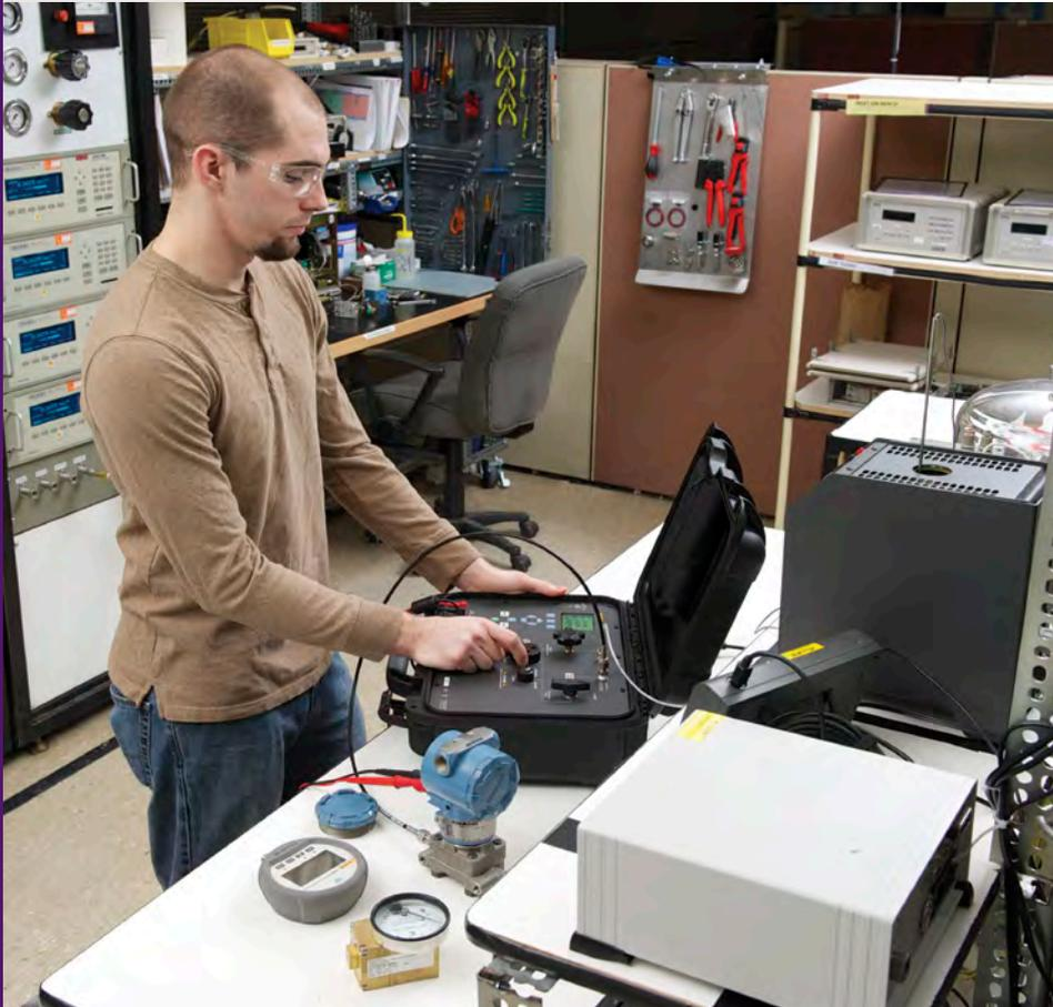
Technicians calibrate at the bench to ensure calibrations are effective and don't result in degradation of performance. They ensure that all components are in good working order prior to installation, and can evaluate them when component failure is suspected. The bench provides a stable ambient environment for calibration, an opportunity to use the most accurate equipment, and protection from factory conditions during the commissioning, testing, and calibration of pressure transmitters.
