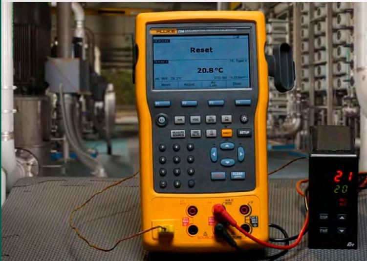
Temperature switches and controllers are commonly used in small processes and in control loops where a programmable logic controller (PLC) or larger distributed control system (DCS) are not warranted.
