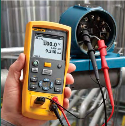
Thermocouples and RTDs are the most common sensors used in process temperature measurements.
