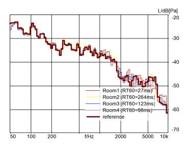
The reference is a recording via the microphone of the DUT in a typical test room. The other four graphs show the recreation of the reference signal by 3PASS lab in four different rooms with different reverberation times. The very high correlation with the reference signal demonstrates the accuracy of 3PASS lab and its automated digital equalization across different laboratories and test rooms.
