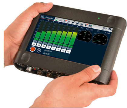
Mobile recording & playback system SQuadriga III
