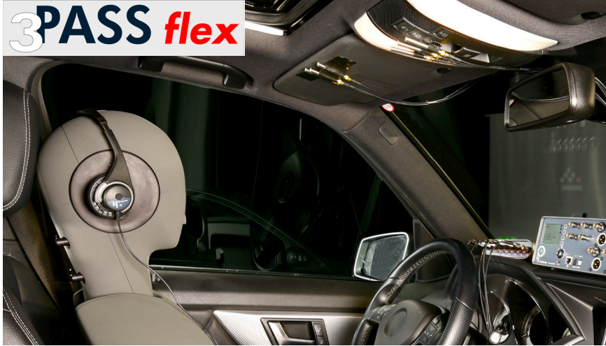
Exemplary custom microphone arrangement for 3PASS flex application in a car
