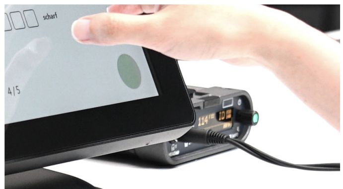
Using the playback module labP2, for example, the original sound spectrum and the spatial distribution of the sound field can be reproduced accurately. labP2 can be cascaded and is the ideal device for the use in listening studios, too.
