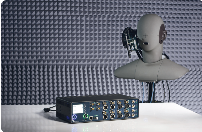
VoIP measurement scenario with HMS II.3, HHP IV and labCORE
