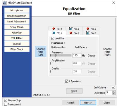
The EQ wizard of HAE-BGN guides the user through the equalization procedure. The system uses a combination of FIR and IIR filters (see screenshots) to equalize the loudspeaker setup
