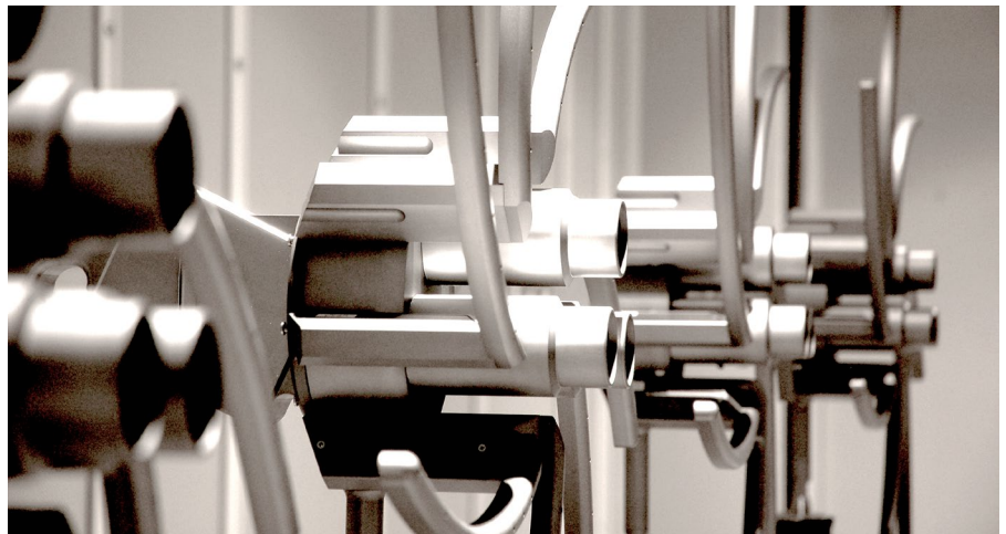
MultipleEye technology: Three synchronously recording cameras allow the exact distance to any object in view to be determined at any time.
