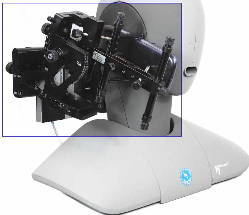
HHP III.1 mounted to artificial head HMS II.3 for voice quality test of 4G smartphone
