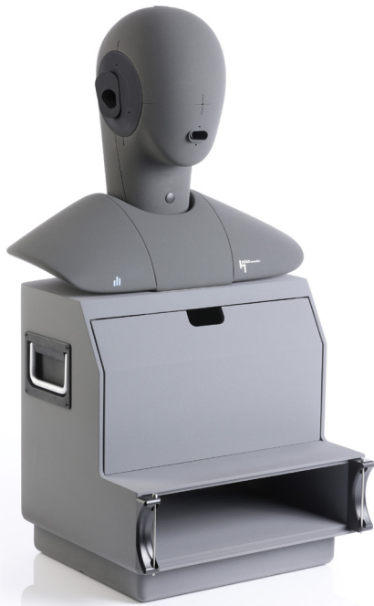
HMS II.6 mounted on the supplied torso box HTB VI (above), exemplary measurement setup in a car (right)
