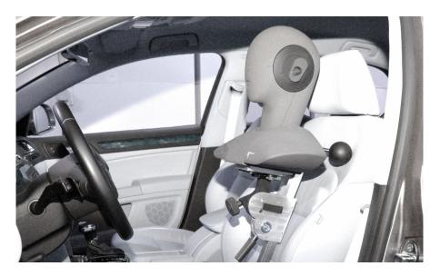
The HSM V seat mount adapter is a stable platform for performing measurements in a vehicle. Thanks to a quick-lock coupling, the HSU III can be attached quickly and easily to the lockable carriage on the back rail, resulting on a position resembling a person sitting in the vehicle.
