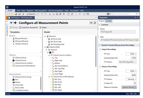
Executing airborne volume source measurements, the measurement points for the microphones, the volume source positions and the airborne receivers can be clearly arranged.
