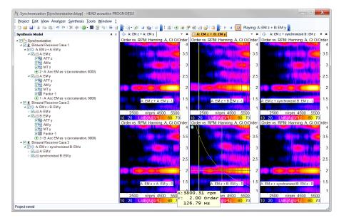
Reinforcements and cancellations (in the 2nd motor order), caused by a superposition of non-synchronous input data, can be prevented by synchonizing via order synthesis.
