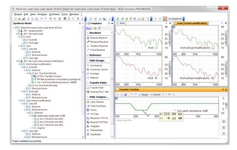
Even large models can be be managed easily with PROGNO[I]SE. Various tools are available for editing, e.g., for smoothing and inverting of transfer functions.
