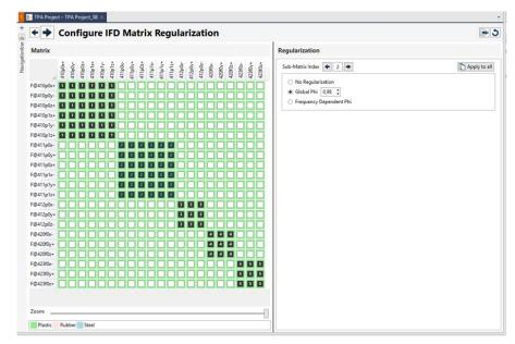
In order to prevent that small measurement errors in the input data lead to an overestimation of path contributions resulting in case of badly conditioned matrices, matrix inversion with frequency-dependent regularization are used.
