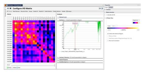
The Mosaic View visualizes the magnitude or the phase of the transfer functions in form of a frequency-dependent, color-coded matrix. This makes it easier for users to gain a profound understanding of systems and provides an aid to decision-making, whether coupling between subsystems must be considered or can be neglected.
