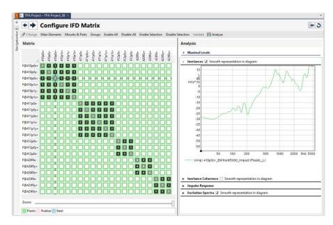
Immediately, the bar display and various diagrams allows the user to check the properties of the impact measurements visually. Subsystems can be independently considered. For that, the associated submatrices are calculated individually and configured independently from each other.
