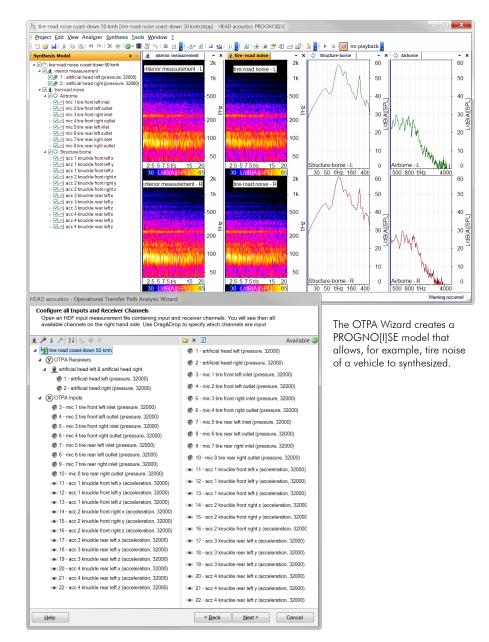
In the OTPA Wizard, the model can quickly be configured from the channels of a measurement.
