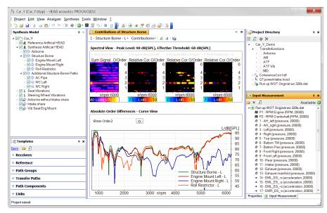
The Contribution Viewer shows the summed signal and all direct sub-elements by means of particularly prepared order spectra (upper diagrams). Also the representation of the order cuts (lower diagram) allows the quick identification of prominent noise components.
