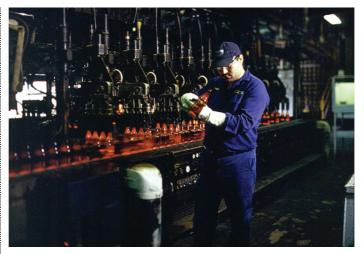
Inspection time: A factory worker manually inspects a rejected glass bottle from the production line. A dataTaker DT80 soon established the production faults leading to these rejects.
