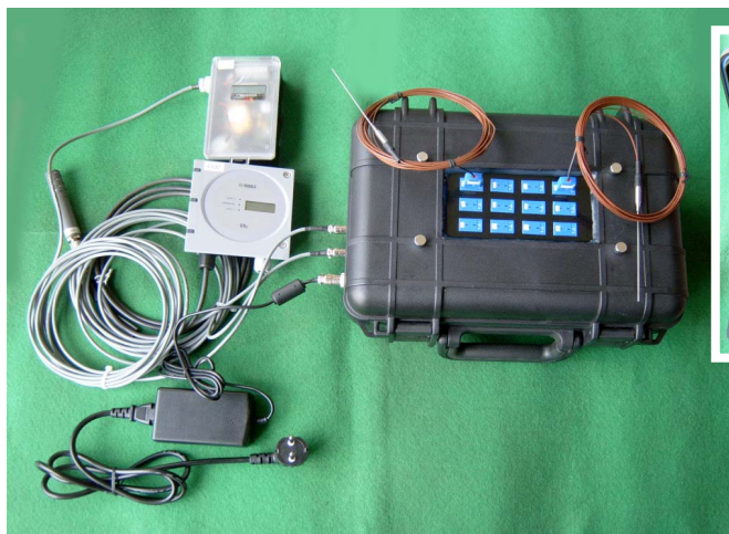
dataTaker enclosure: The DT80 is safely mounted and powered from within the enclosure so as to mitigate risk of damage or tampering
