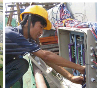
An integrator sets up the dataTaker logging system, which monitors the structural integrity of the National Gymnasium
