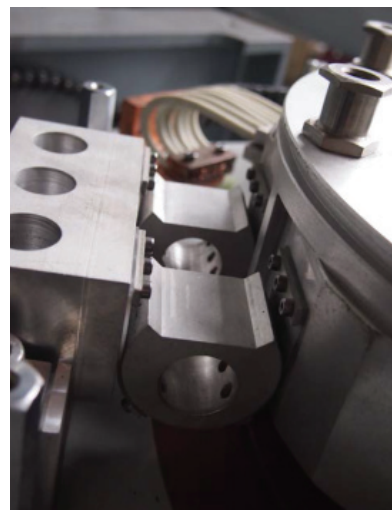
Left - Rolling link "dog bone" used in longer stroke machines is entirely metallic.
