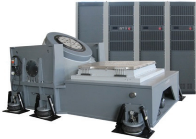
A typical high-force water-cooled system including a shaker and mono-base slip-table with air isolation mounts.
