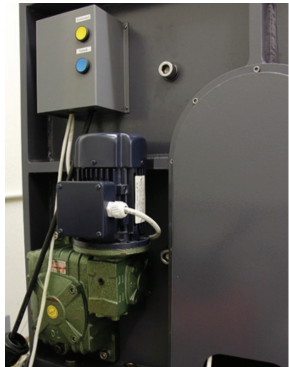
Optional motorized gearbox for shaker rotation.
