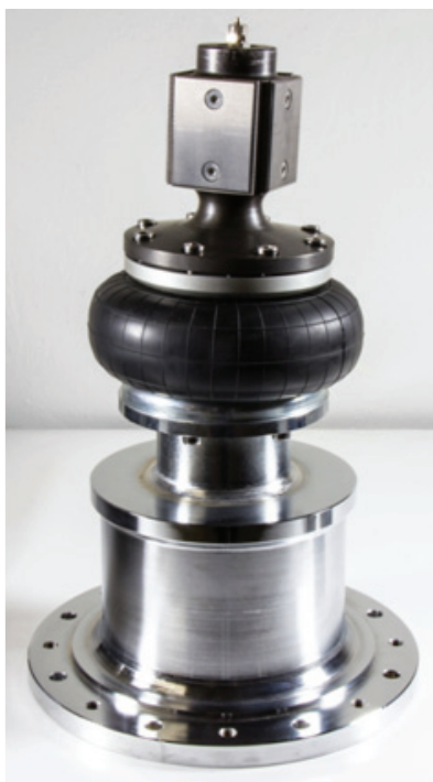
Lower suspension square guidance post sitting on air-spring over air chamber and base attachment plate. The post is held to the armature by a screw.
