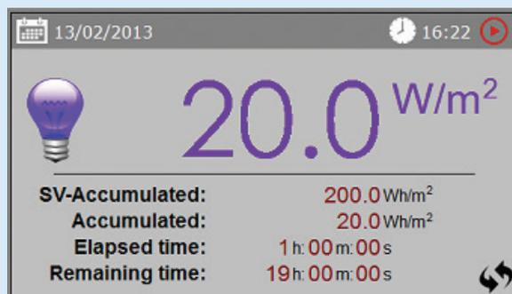
ClimaPlus controller specific for Photostability chambers with automatic integration of VIS and UV sensors and light meters according to traceability standards. Enables automatic running (with auto-stop) of test programs and FDA 21 CFR compliant data logging.
