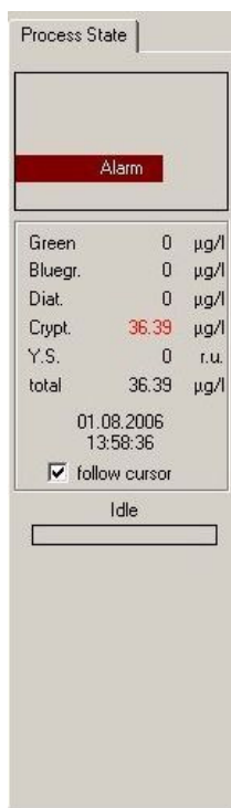
Alarm indication in AOA software when operating via PC
