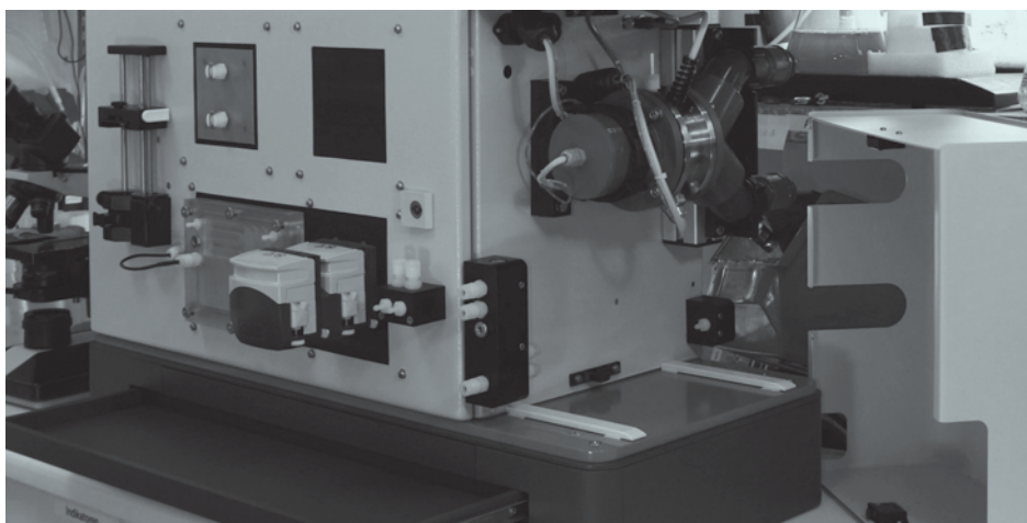
Daphnia Toximeter II with drip pan, pumpheads and filter unit
