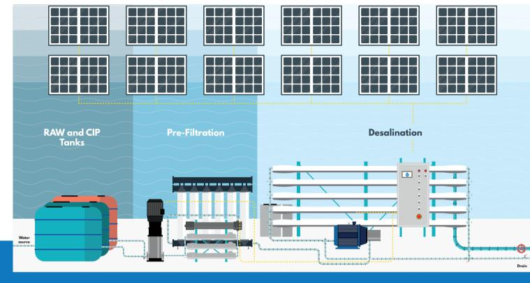
The Systems runs 100% on solar energy. No external power source or power buffer is needed, resulting in the perfect island solution.
