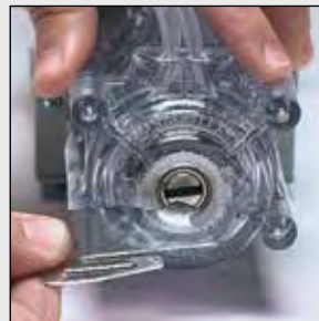
3. Reassemble two halves and mount on drive.
