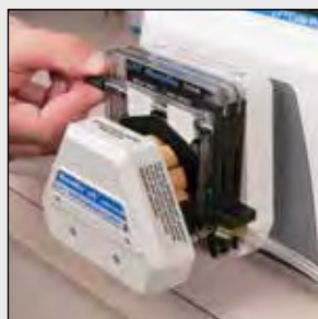
3. Adjust occlusion using index scale on cartridge.
