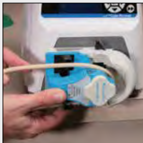
2. Place tubing over rollers and through retainers.
