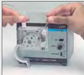
2. Hook left-side tubing stop to the top of the left-side retainer slot. Stretch tubing around rollers and hook right-side stop to the top of the right-side retainer slot.
