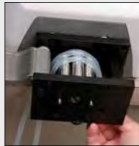
3. Stretch tubing and hook right side stop underneath retainer slot. Close and latch occlusion bed.
