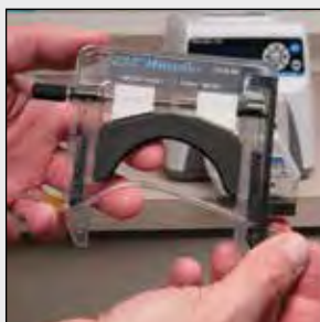
1. Select tubing, load cartridge, and set tubing retainers.
