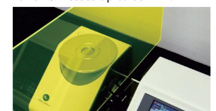
For liquids, optional cells with 3 optical path lengths for different sample densities are available, and commercial 10 mm-wide cells can also be used.
