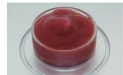
Colorant pellets can be measured in raw form using a Petri dish (optional accessory).
