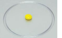
Pastes can also be measured using a Petri dish (optional accessory).
