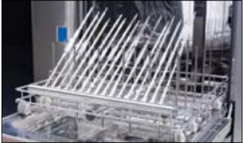
Pipets may be thoroughly washed and dried in FlaskScrubber and FlaskScrubber Vantage Series Washers. Pipet Inserts attach to the spindle rack to allow the interior of the pipets to be injected with water and detergent for washing followed by hot air for drying.
