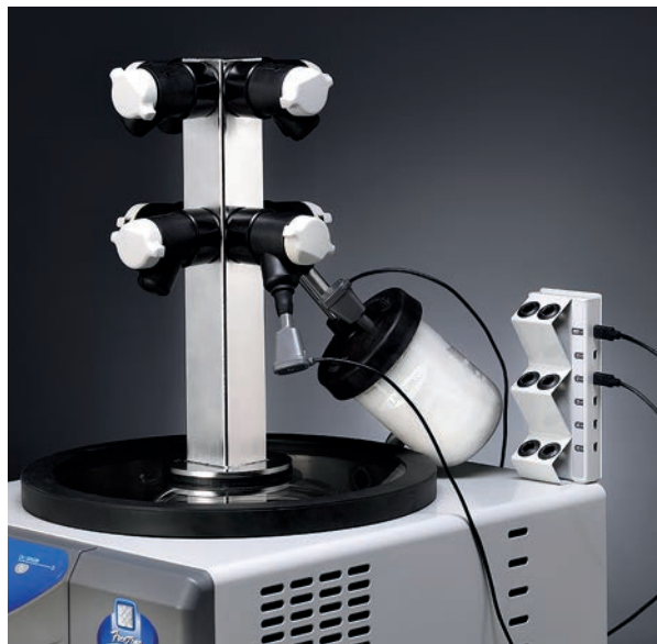
End-Zone Starter Kit 780901000 is shown connected to FreeZone 4.5 Liter Benchtop Freeze Dryer 700401000 with 8-Port Manifold 7201800
