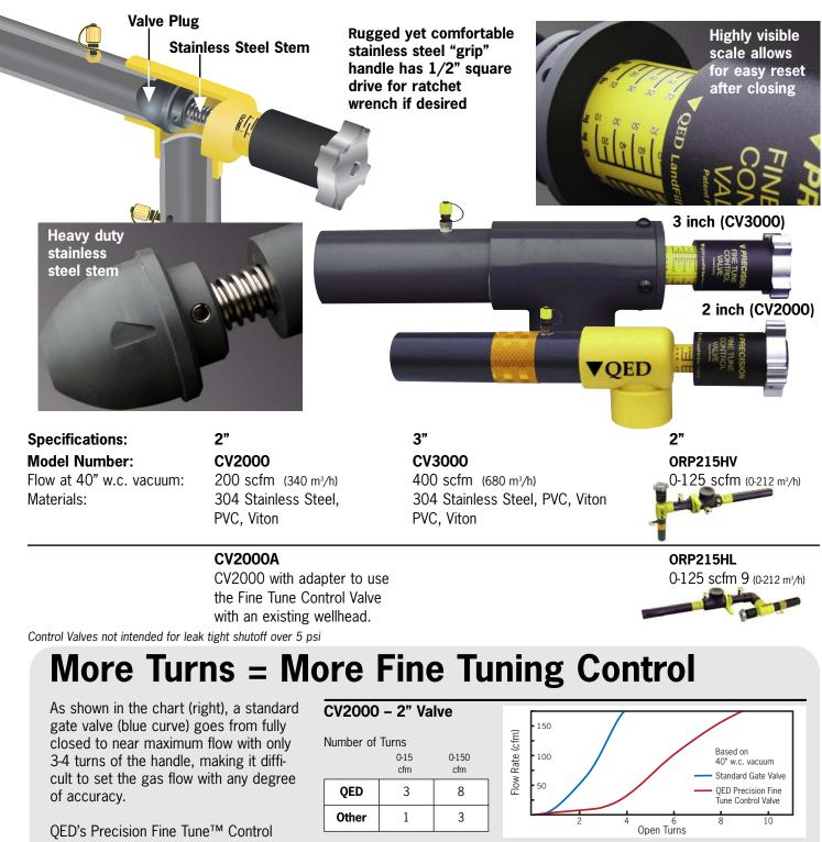
Valve (red curve) takes 9+ turns to go from fully closed to near maximum flow, making flow adjustment far more linear. Because QED's valve requires more turns to achieve a given flow rate change, it allows the operator to make more precise adjustments. This is especially true at lower flow rates.
