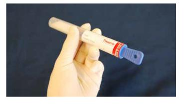
Sample using a back and forth motion within sampled area.
