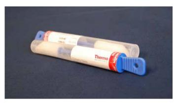
2. Grip handle of swab and gently twist to break tamperevident seal. Pull handle slightly to remove Environmental Flexi Swab from transport tube.
