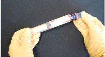
4. Return Environmental Flexi Swab to its original transport tube. Ensure that transport tube is labelled.
