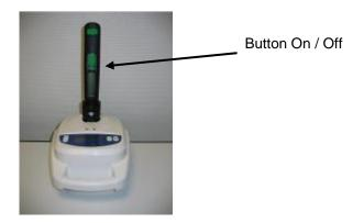
Start the Coriolis<sup>®</sup>µ at 300l/min and wait until the speed becomes stabilized (10 to 15 seconds).
