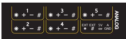
Figure 2: DT80 analog terminals
