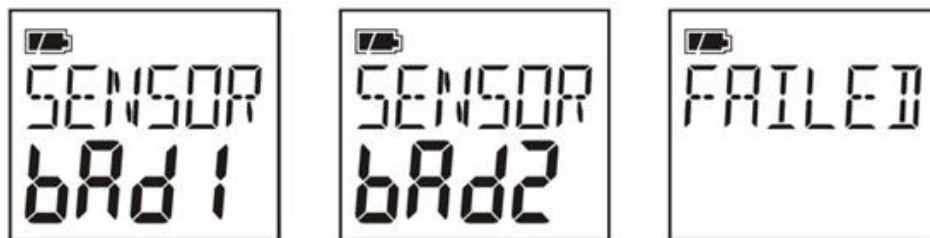
Figure 24: Display of Failed Calibration
