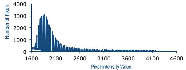
**Figure 6:** Intensity histogram for sCMOS. Courtesy of Y. Sabharwal; Reproduced from *Microscopy and Analysis* 26 (1), January 2012, Copyright 2012 John Wiley and Sons Ltd.
