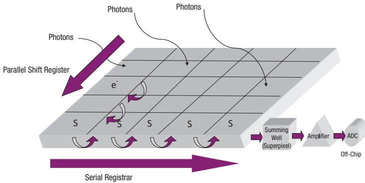
**Figure 2:** Readout of a CCD chip 4 x 4 pixel array. Row labelled with “S” indicates the serial register. Other pixels are part of the parallel shift register. After (summing if binning) and amplification, the signal moves off-chip and is then converted from analog to digital via the analog to digital converter (ADC).
