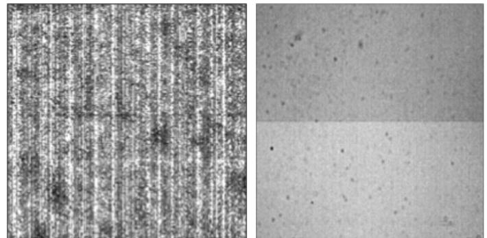
**Figure 9:** (Left) Column to column variation due to multiple column amplifiers of sCMOS. Reproduced with permission from Photometrics. (Right) Manifestation of bi-directional readout of sCMOS chip. Courtesy of Y. Sabharwal; Reproduced from *Microscopy and Analysis* 26 (1), January 2012, Copyright 2012 John Wiley and Sons Ltd.
