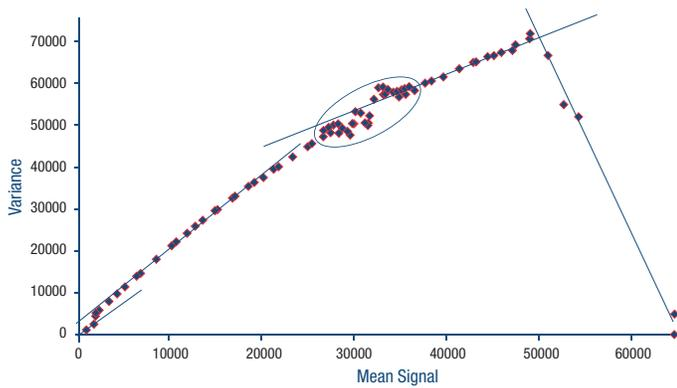
**Figure 5:** Mean-variance curve for sCMOS. Courtesy of Y. Sabharwal; Reproduced from *Microscopy and Analysis* 26 (1), January 2012, Copyright 2012 John Wiley and Sons Ltd.
