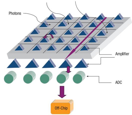
**Figure 3:** Readout of sCMOS chip. Each pixel has its own amplifier, and each column has its own amplifier and analog-to-digital converter (ADC). Readout is done on the chip, through multiple ADCs, thereby improving readout speed.
