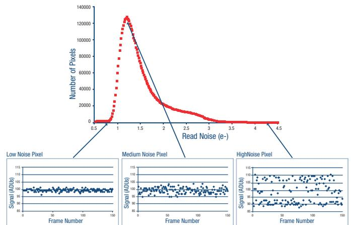
**Figure 8:** Non-gaussian, positively-skewed distribution of sCMOS sensor. Variability of noise among different pixels. Courtesy of Y. Sabharwal, J. Joubert, and D. Sharma; Reproduced from *Microscopy and Analysis* 25, published online September 2011, Copyright 2011 John Wiley and Sons Ltd.
