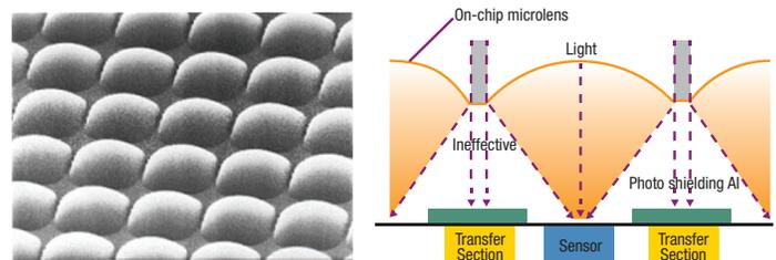
**Figure 4:** Microlens array (left). Light redistribution from non-photosensitive regions to photosensitive regions (right). Reproduced from King Leader, “Frequently asked questions,” <http://www.kl-security.com/technology/faq/>. Accessed 09/20/2012.
