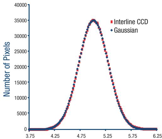
**Figure 7:** Gaussian distribution of read noise for CCD sensor. Courtesy of Y. Sabharwal, J. Joubert, and D. Sharma; Reproduced from *Microscopy and Analysis* 25, published online September 2011, Copyright 2011 John Wiley and Sons Ltd.
