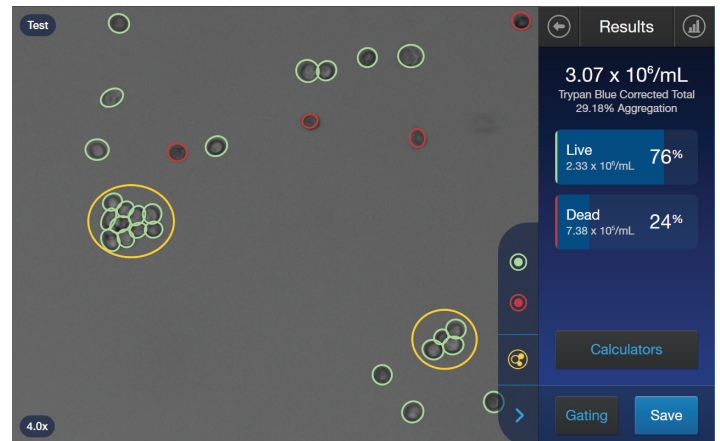
Figure 3. Accurate cell counts, even with clumpy samples. The segmentation and counting algorithms of the Countess 3 cell counter were able to resolve clumps in this U2OS human osteosarcoma cell sample and show the percent aggregation within the sample.
