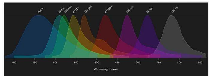
**Figure 2. Fluorophore emission spectra of primary antibody conjugates in a 9-plex panel.** The relative fluorescence intensity for each fluorophore in the 9-plex panel is plotted by wavelength. The spectra display extensive overlap, which requires spectral unmixing to resolve.
