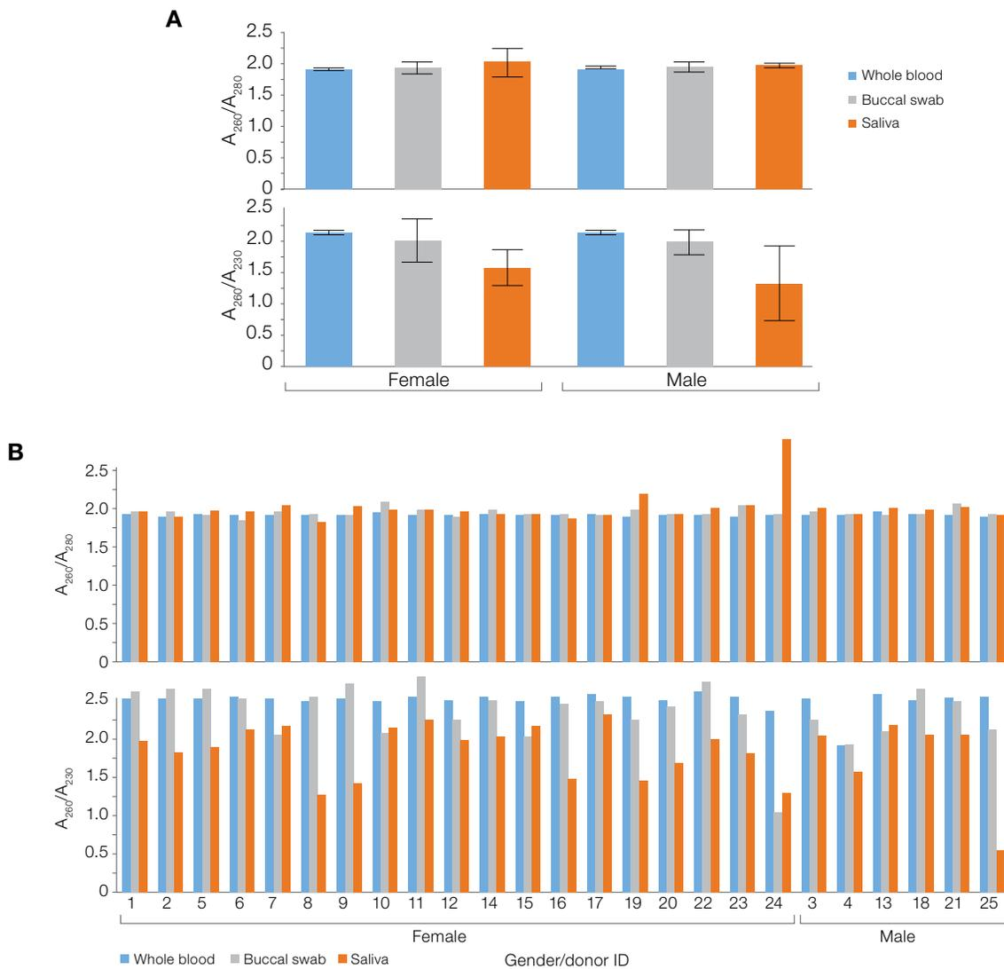
**Figure 3.**  $A_{260}/A_{280}$  and  $A_{260}/A_{230}$  values obtained with the NanoDrop 8000 Spectrophotometer across whole blood, buccal swabs, and saliva samples. (A) Average values by gender and (B) individual values for all samples.
